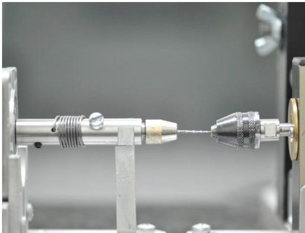
Fig. 5. Ni-Ti instrument clamped between the chucks.
