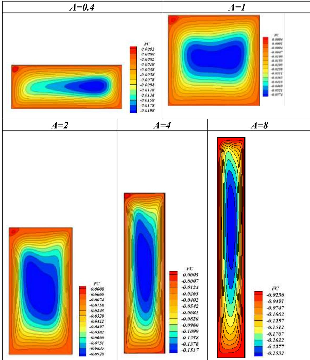
Fig. 3 Stream function for  $Ra=10^5$  and  $A=[0.4, 1, 2, 4, 8]$
