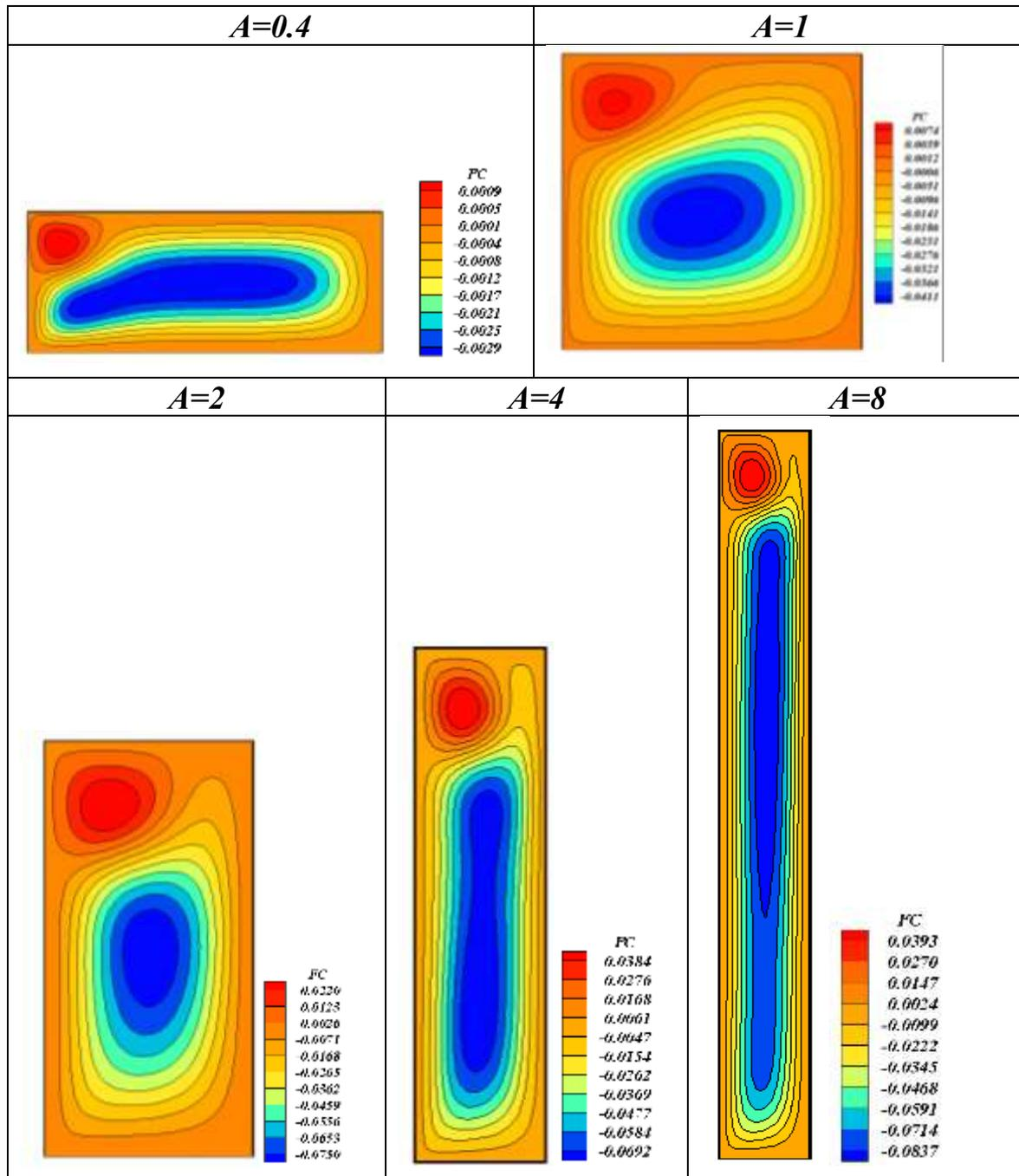
Fig. 2 Stream function for  $Ra=10^4$  and  $A=[0.4, 1, 2, 4, 8]$
