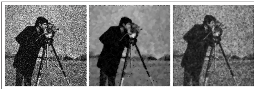
Figure 6. Cameraman image affected by Gaussian noise with variance 50 (left image), restored with our filter (middle image) and restored with the Wiener filter using 5 \times 5 neighbours (right image). The values of PSNR and MAE of our method are, respectively, 18.87 and 20.16, while those achieved by the Wiener filter are, respectively, 12.05 and 63.65.
