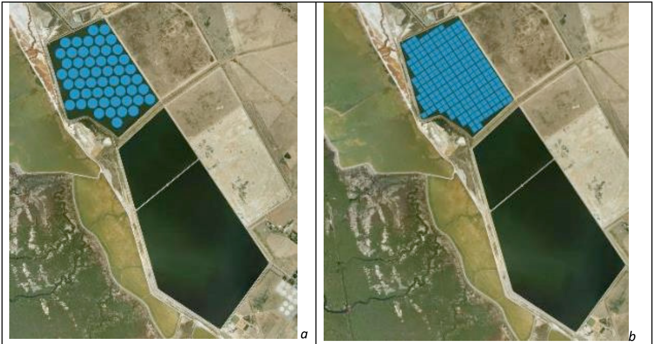
Figure 4 A schematic drawing of two different solutions for Bolivar wastewater basin.
