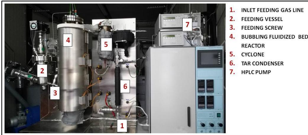
FIGURE 2. BFB bench-scale gasifier
