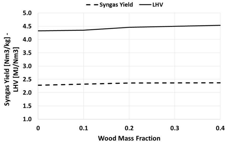
FIGURE 4. Sensitivity analysis of syngas heating values and syngas yield at 750°C and S/B=0.5
