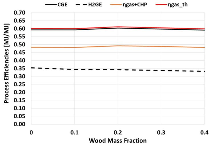
**FIGURE 5.** Sensitivity analysis of cold gas efficiency (CGE), gasification thermal efficiency ( $\eta_{gas\_th}$ ), hydrogen gas efficiency (H<sub>2</sub>GE) and electrical efficiency (EE) for gasification coupled with a CHP unit (reciprocating engine, efficiency 37.5%)
