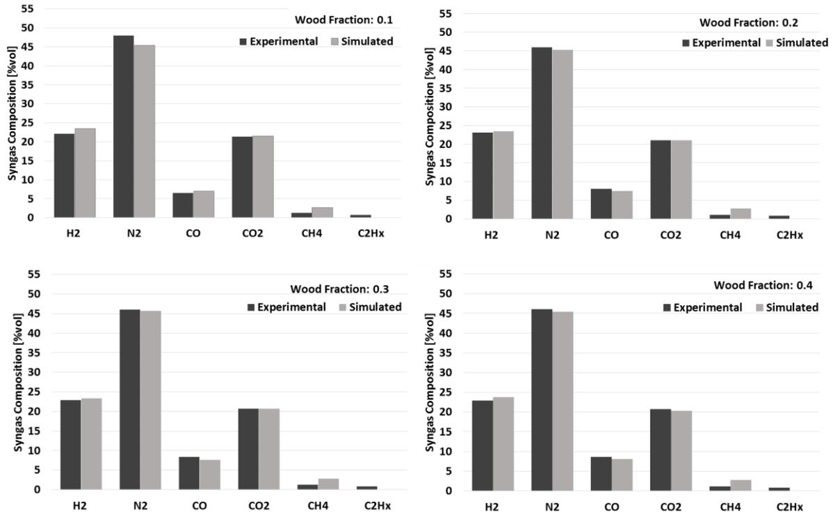
**FIGURE 3.** Simulation model validation by syngas composition at different wood mass fraction (0.1, 0.2, 0.3, and 0.4). Black columns experimental data, grey columns simulated data.
