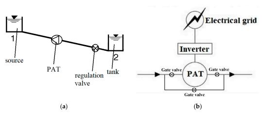
**Figure 1.** Example of transmission main (**a**). Layout of pump as turbine (PAT) installation, adapted from [11] (**b**).
