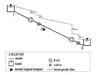
**Figure 6.** Layout of the system of transmission mains of S. M. La Stella. Qualitative pattern for the head grade line for the solution with  $C_{inst,tot} = 12,021 \in$  and  $P_{PAT,tot} = 8.74$  KW. See Table 3 for numerical values.
