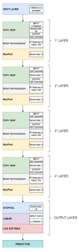
Figure 3. Convolutional neural network architecture.
