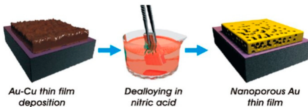
Figure 2. Schematic picture of the free-corrosion dealloying process of Au-Cu alloy film for the production of NPG film. Reproduced with permission from [39]. Copyright American Chemical Society, 2015.
