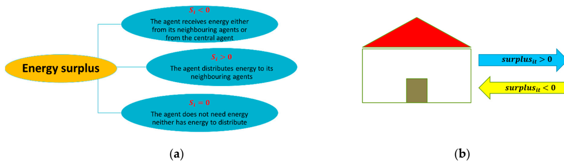
Figure 1. (a) Distribution patterns established on the grounds of the value of the surplus_{it} ; (b) Direction of the energy exchange in accordance with the sign of the surplus_{it} .
