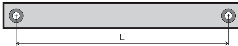
Figure 4. Layout of a cable: The construction length L_0 is affected by manufacturing errors generated during the cutting operation and assembly errors coming from a bad placement of the eyelets necessary to connect two or more cables.
