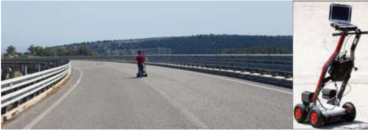
Fig. 2. Ground coupled GPR survey during the bridge monitoring.
