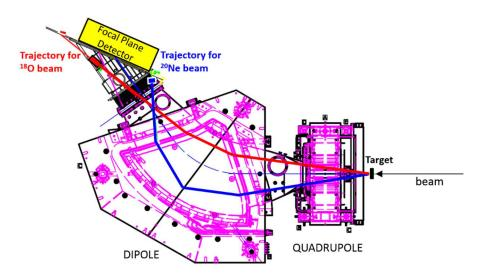
Fig. 1. Drawing of the MAGNEX spectrometer showing two typical trajectories of the <sup>18</sup>O and <sup>20</sup>Ne beams in the experimental conditions used for the DCE measurements.
