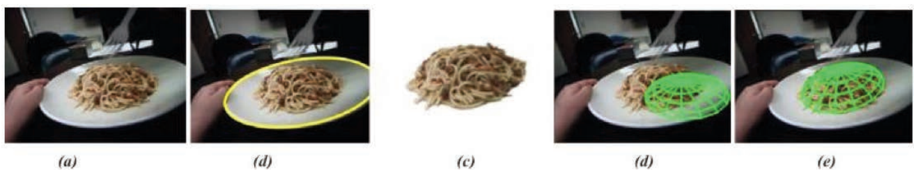
Figure 7. Image processing performed in Sun et al. (2014): a) input image, b) plate detection, c) food segmentation, d) shape modelling and e) shape fitting.
