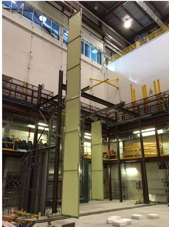
Figure 3.22. A 12 m DUNE-SP CPA mock-up panel (foreground) and a half-height 6 m ProtoDUNE-SP panel mock-up (rear) at Ash River, Minnesota.
