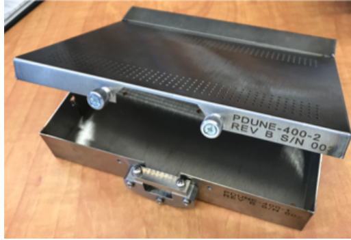
Figure 4.25. Prototype CE box used in ProtoDUNE-SP.
