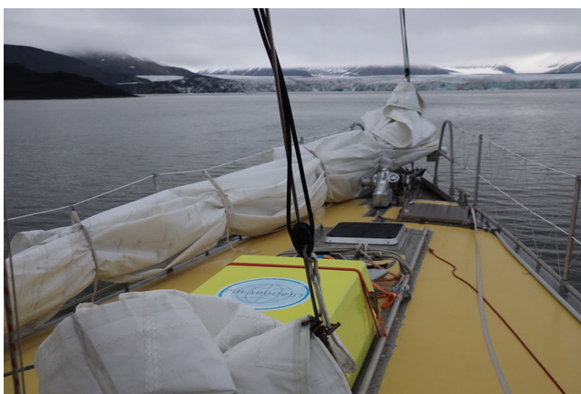
Figure 3. Photo of the POLA-01 detector enclosed in its fiberglass yellow hutch on the deck of the Nanuq sailboat. (Photo by O. Pinazza).
