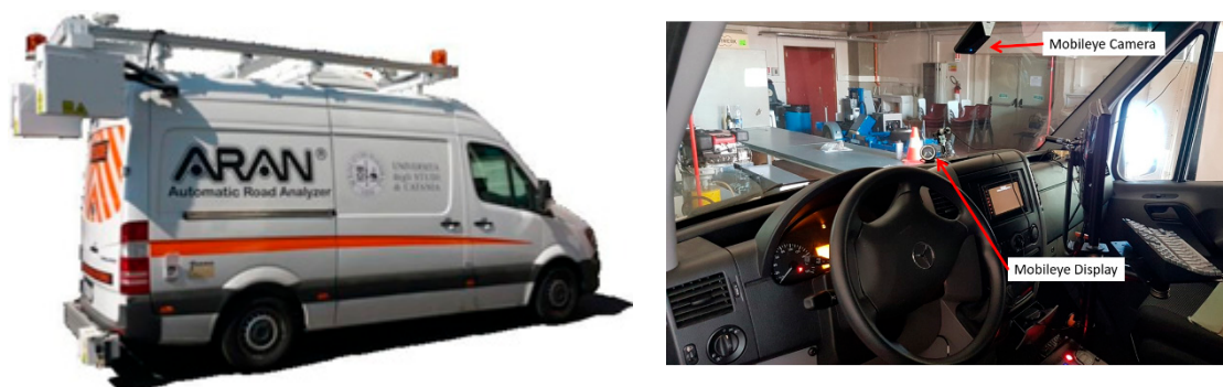
Figure 1. Mobileye 6—in-vehicle installation.
