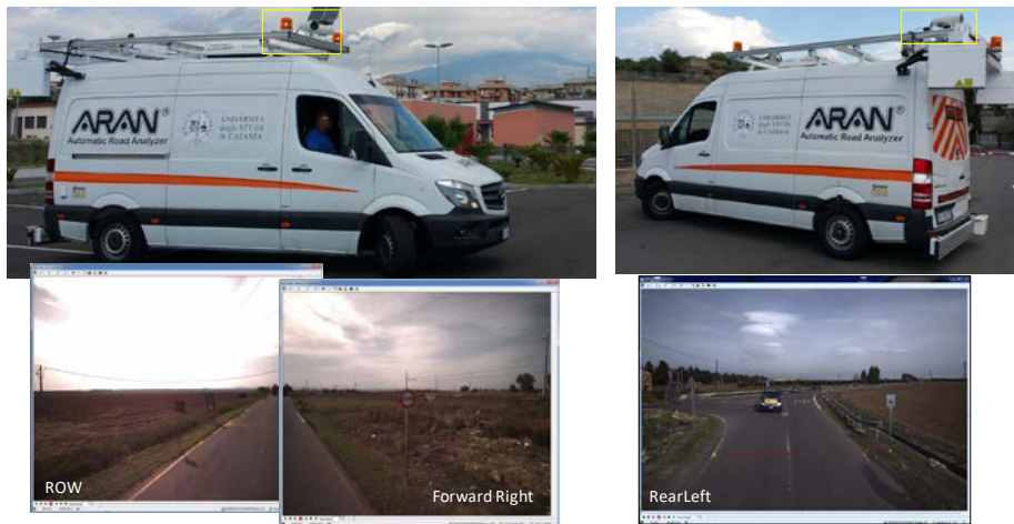
Figure 3 Road Video Survey.
