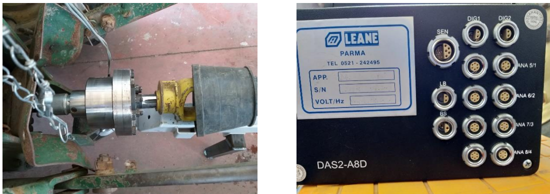
Figure 2. (a) The torque-meter connected to the power take-off (PTO); (b) The acquisition system of the torque-meter.
