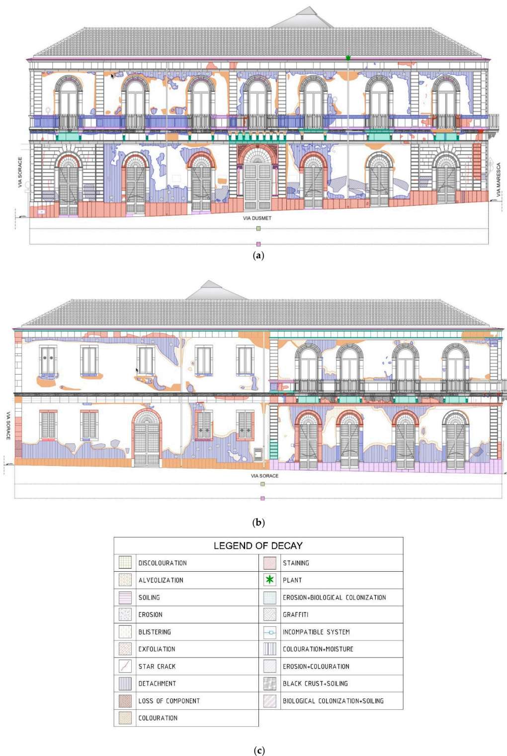
Figure 10. (a) Decay mapping on eastern façade; (b) Decay mapping on southern façade; (c) Legend of detected decay.
