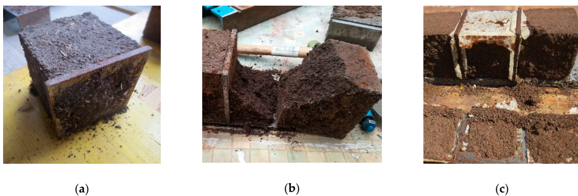
Figure 2. Some documented cases of loss of integrity, despite the following treatments: (a) sanding; (b) water film; (c) parchment paper.
