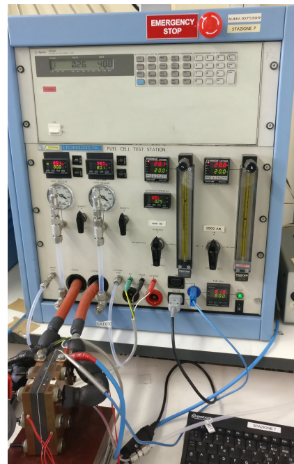
Figure 4. Fuel Cell Technologies Testing Station (FCT-TS) used in experiments at CNT-ITAE laboratories.
