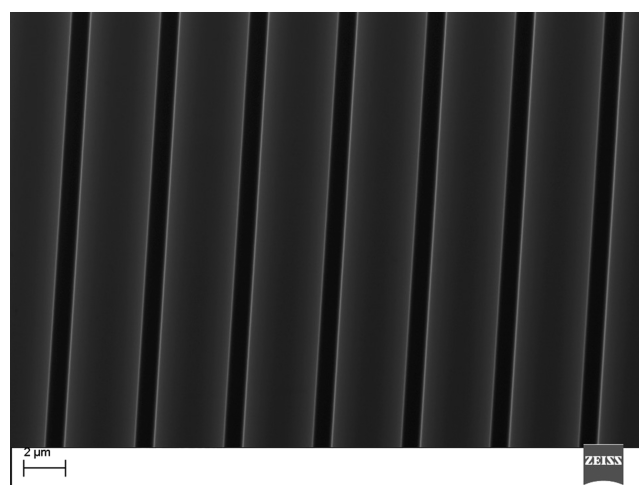
Figure 2. In-plane view of the SEM analysis of the trenches in the SiC wafer after the HF + NH_4F treatment.
