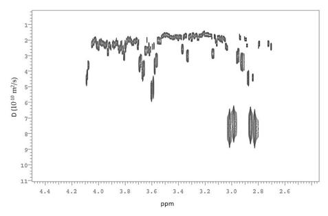
**Figure 7.** DOSY spectrum of lemon-PEI CDs dispersed in deuterium oxide (D2O). Diffusion coefficient values, D, are reported on the y-axis.
