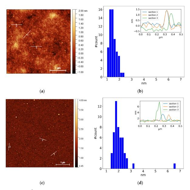
**Figure 2.** (a)  $5 \times 5\mu m^2$  AFM image of lemon-PEI CDs deposited onto silicon substrate (z scale:  $0-20^\circ$ ); (b) histogram analysis of lemon-PEI CDs' height obtained by several sections, three of which are represented in the inset; (c)  $5 \times 5\mu m^2$  AFM image of lemon-only CDs deposited onto silicon substrate (z scale:  $0-20^\circ$ ); (d) histogram analysis of height of lemon-only CDs obtained by several sections, three of which are represented in the inset;
