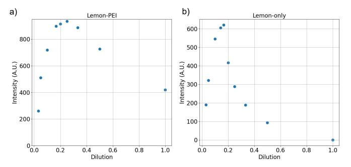
**Figure 5.** (a) Intensity of fluorescence peak as a function of the dilution of an aqueous suspension of lemon-PEI CDs ( $\lambda_{ex} = 340 \text{ nm}$ ,  $\lambda_{em} = 470 \text{ nm}$ ); (b) intensity of fluorescence peak as a function of the dilution of an aqueous suspension of lemon-only CDs ( $\lambda_{ex} = 330 \text{ nm}$ ,  $\lambda_{em} = 440 \text{ nm}$ ).
