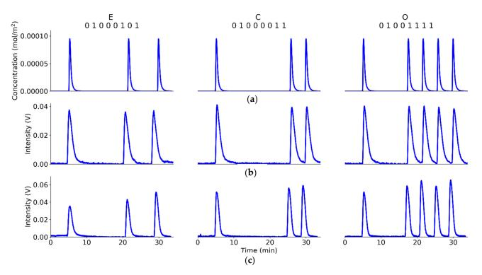
**Figure 8.** (a) Simulated message corresponding to "ECO" word in binary coding (simplified ASCII), obtained by modelling a capillary 0.40 mm in radius and 200 mm in length and setting the RMS velocity of the flow to 5.7 mm/s and the pulse of information particles to a volume of 20  $\mu$ L; experimentally, transmission of the word "ECO" was performed by using (b)lemon-only and (c) lemon-PEI carbon dots, respectively.
