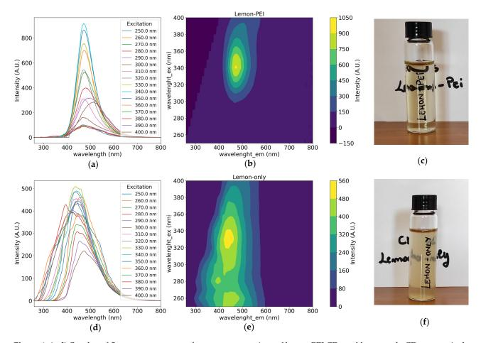
**Figure 4.** (**a**,**d**) Overlay of fluorescence spectra of aqueous suspensions of lemon-PEI CDs and lemon-only CDs, respectively, acquired at several excitation wavelenghts as reported in the labels; (**b**,**e**) excitation–emission maps of aqueous suspensions of lemon-PEI CDs and lemon-only CDs, respectively; (**c**,**f**) photos depicting the qualitative appearance of the aqueous suspensions of lemon-PEI and lemon-only CDs.
