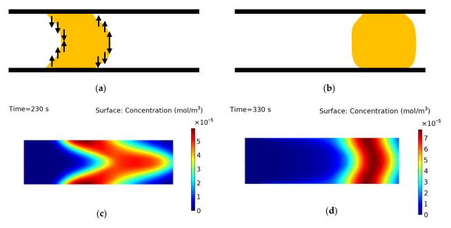
**Figure 6.** (a) Schematic representation of the transversal diffusion following concentration gradients; (b) schematic representation of the effect of the transversal diffusion at high diffusion coefficient; false colour map of simulated molecular messenger concentration distribution with lower diffusion coefficient (c), and with higher diffusion coefficient (d).
