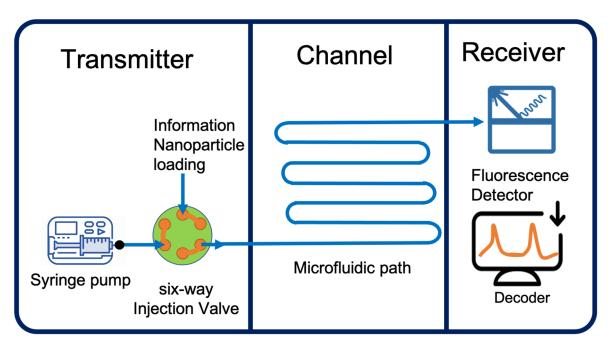
**Figure 1.** Schematic representation of the MoCo prototypal platform applied for communication trough body fluid among implanted biodevices.
