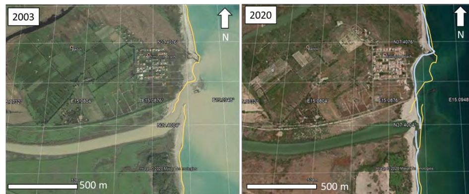
Figure 7. Retreat of the Simeto river mouth on the Catania coastal plain. The shoreline at 2003 epoch is marked in light orange (left) while the shoreline for 2020 epoch is marked in light blue (right).
