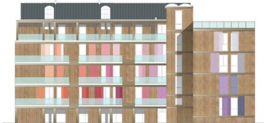
Figure 8. South front of the case study building after the application of prefabricated timber panels clad with wooden boards.
