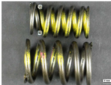
Fig. 4. Valve spring after testing in overspeed condition (breakage on inner spring from bottom side).
