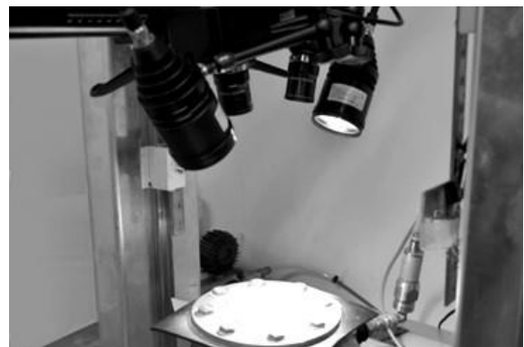
Figure 3. Bulge test setup for 3D-DIC technique (Courtesy of authors [22]).
