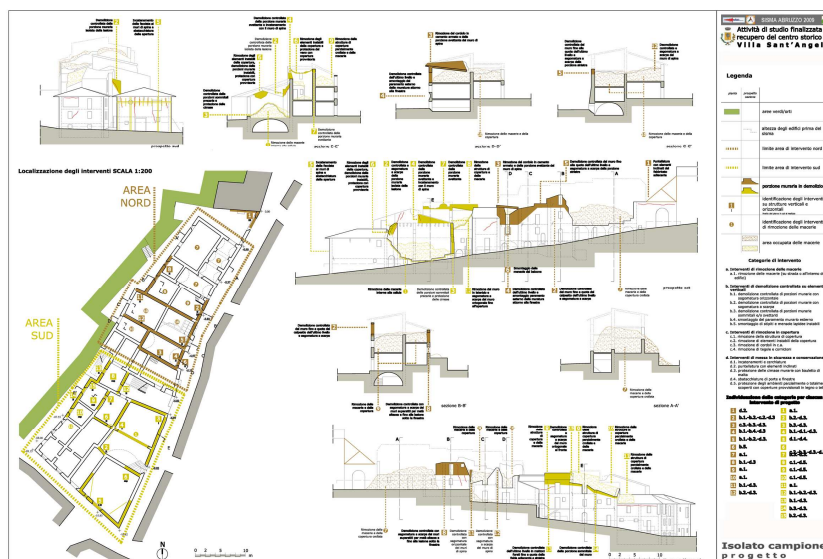
Figure 6: Project state of the sample block
