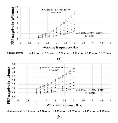
**Figure 17.** (**a**) Power/linear displacement ratio frequency response functions (FRF) and (**b**) Energy/linear displacement ratio FRF.
