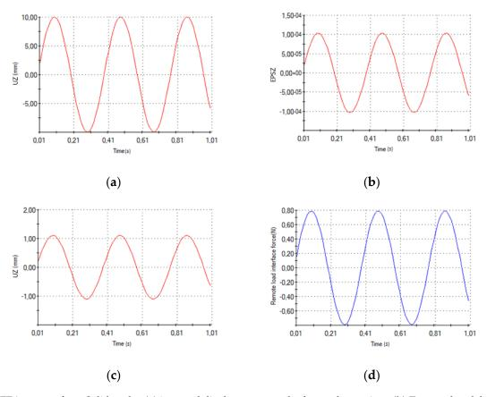
**Figure 9.** FEA screens from Solidworks: (**a**) imposed displacements at the free end over time, (**b**) Z-normal nodal averaged strain on upper PPT surface over time, (**c**) displacements along Z-axis at 100 mm from fixed joint cross-section over time, and (**d**) nodal averaged reaction force along Z-axis at 100 mm from fixed joint cross-section.
