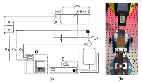
**Figure 11.** (a) Setup scheme (signal generator and amplifier (*I*), data acquisition system (*O*), linear displacement signal ( $o_1$ ), load cell signal ( $o_2$ ), PPT signal ( $o_3$ ), probe (*Z*), resistor (*R*)), and (**b**) experimental setup.
