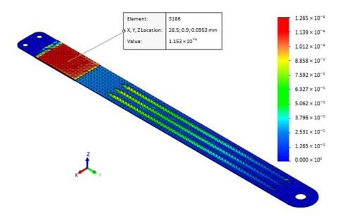
**Figure 10.** Z-axis normal strain corresponding to maximal imposed displacement. The measurement unit is mm/mm.
