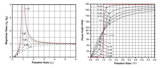
**Figure 3.** Magnitude ratio and phase of the response of a typical mass-spring-damper as a function of  $\lambda$ .
