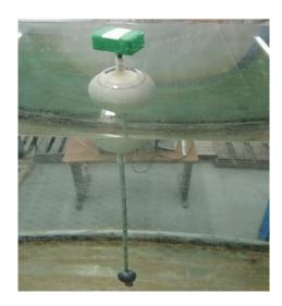
Figure 6. Spar buoy scaled model during test.
