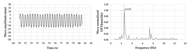
Figure 7. Wave amplitude and normalized DFT in artificial channel.
