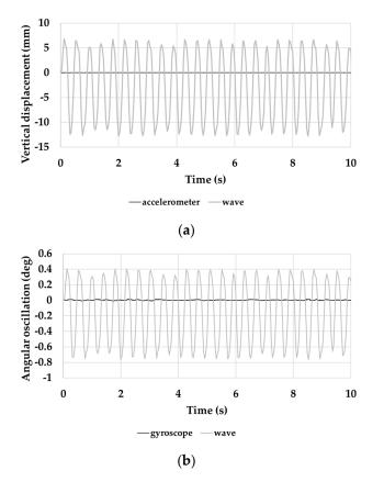
**Figure 15.** (**a**) comparison between the vertical displacement measured by accelerometer along the Z-axis and the wave magnitude; and, (**b**) comparison between the angular oscillation measured by gyroscope around X-axis and the oscillation occurred by the wave.
