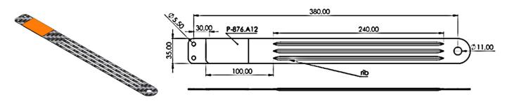
Figure 8. Geometrical characteristics of the deformable band.
