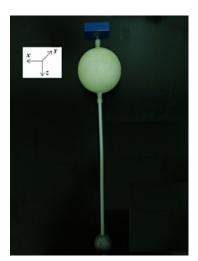
**Figure 1.** Spar buoy scaled model at "fixed-point" test configuration.
