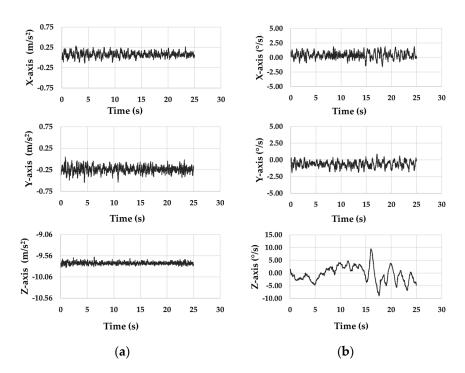
Figure 12. Signals from (a) accelerometer and (b) gyroscope of iNEMO inertial module.
