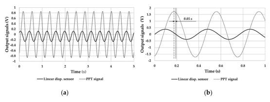
**Figure 13.** (**a**) Harvester and linear displacement sensor signals over time and (**b**) sinusoidal laws of outputs from PPT and displacement sensor.
