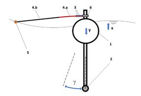
**Figure 2.** Scheme of the energy conversion apparatus for the Lab on sea unit: 1. spar buoy; 2. ballast; 3. piezoelectric patch transducers (PPTs); 4. band (a) deformable part, (b) rigid part; 5. external float; and, 6. rod grip. The vertical direction of the wave motion is indicated with *x*, while *y* is the vertical displacement of the spay buoy and  $\gamma$  is its angular oscillation.
