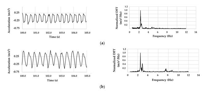
Figure 4. Comparison between acceleration and normalized DFT (a) at sea and (b) in artificial channel.
