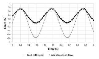
Figure 14. Comparison between load cell output and FEA computed reaction force.
