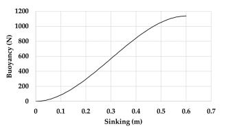
Figure 5. Buoyancy-sinking curve for the spar buoy.
