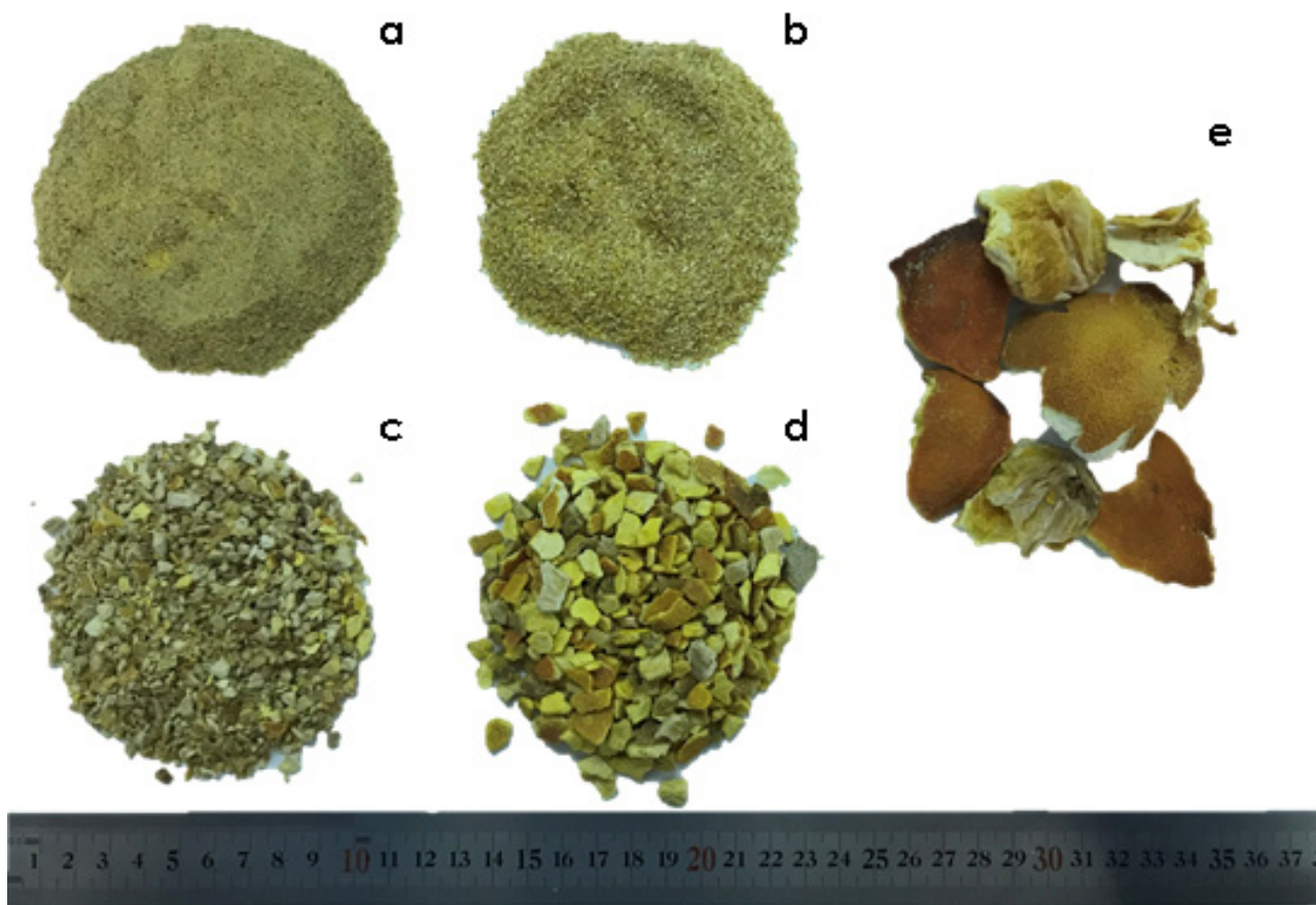
Figure 3. Particle size distribution obtained from sieving (a) s < 0.63 mm; (b) 0.63 < s < 1.25 mm; (c) 1,25 < s < 4.00 mm; (d) s > 4.00 mm; (e) dried citrus peel.
