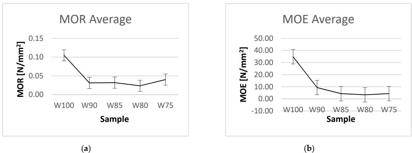
Figure 9. Flexural (a) strength and Modulus of elasticity (b) for the blends.
