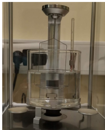
Figure 4. Balance for density determination.
