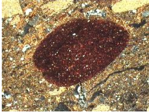
Plate 21. Fabric 5a Fine Clay Component of Clay Mix (Width of Image = 2.5mm)
