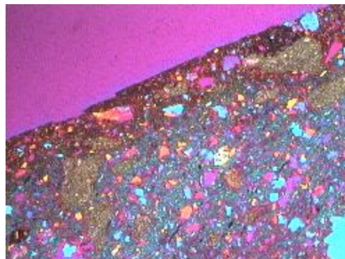
Plate 26. Fabric 5a (98/63) Compacted Surface Layer Viewed with Lambda Plate (Width of Image = 2.5mm)
