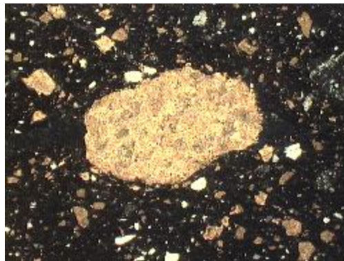
Plate 20. Fabric 2a. Micritic Clot Exhibiting Relict Primary Texture (Sparite) (Width of Image = 2.5mm)
