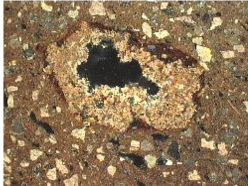
Plate 19. Fabric 1c. Micritic Clot with Red Ring (Iron Migration) (Width of Image = 2.5mm)
