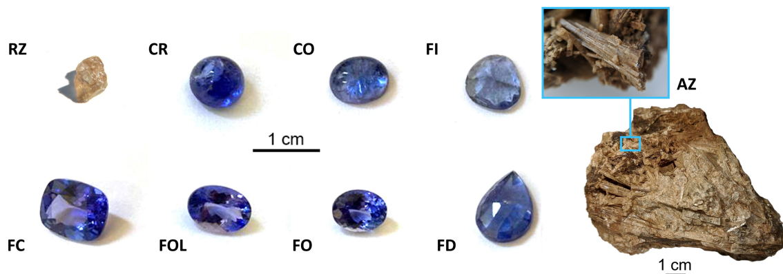
FIGURE 1 Photographs of the analysed samples and detail of the AZ crystals used for polarized Raman measurements
