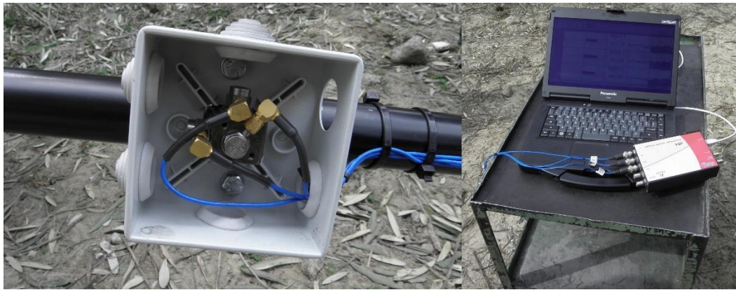
Figure 3. The accelerometers on the rod and the PC-based signal acquisition system.
