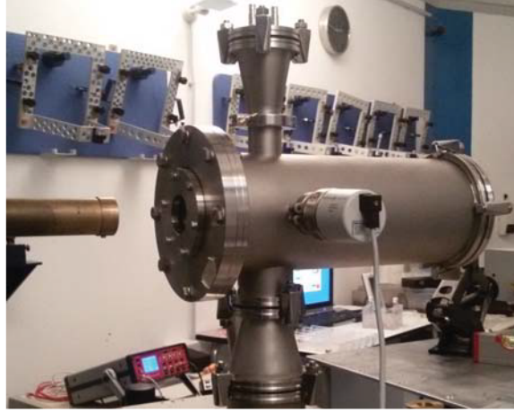
Figure 3.1: The Faraday cup with its line support opened.
