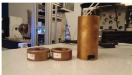
Figure 4.7: The three brass collimators used for the measurements, from left 20 and 25 mm of diameter and, the longer one, the 20 mm diameter antiscattering collimator.
