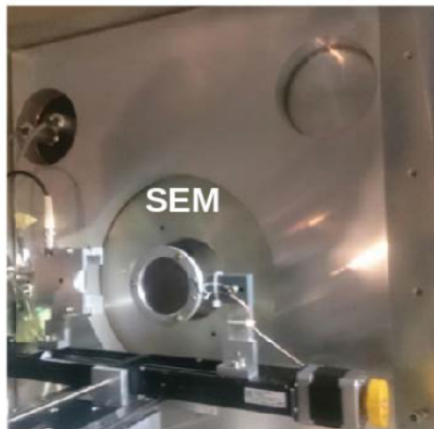
Figure 5.10: SEM placed at about 70 cm from the target and about 10^\circ with respect to the target normal direction, inside the target chamber.
