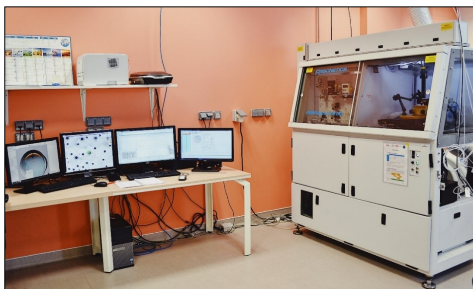
Figure 11: Resonetics M-50 Excimer Ar/F laser ablation (Laboratoire Magmas et Volcans Clermont-Ferrand, France).
