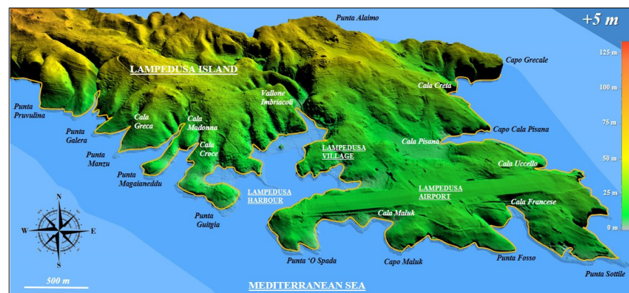
Figure 8. 3D flooding map (+5 m) along the southeastern sector of the island of Lampedusa.
