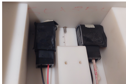
Figure 3.10: Hosted in the center of the shield, right in front of the hole corresponding to the vertex of the exit cone are placed the ^{252}\text{Cf} source and the deployed tagger scintillators.
