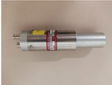
Figure 3.17: One of the plastic scintillators EJ-276 used in the neutron spectrometer.
