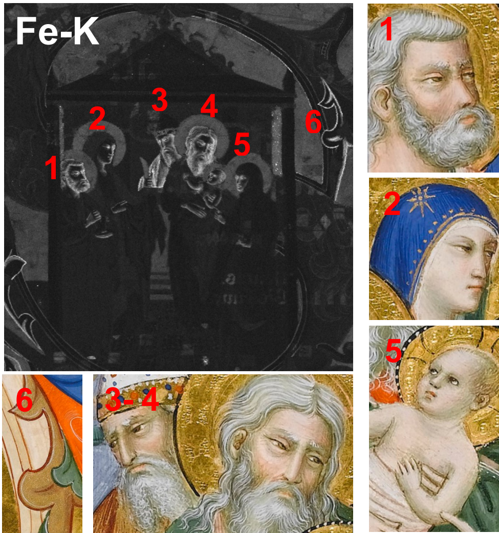
Figure 103: Fe-K image and pictorial details characterized by the ochres presence
