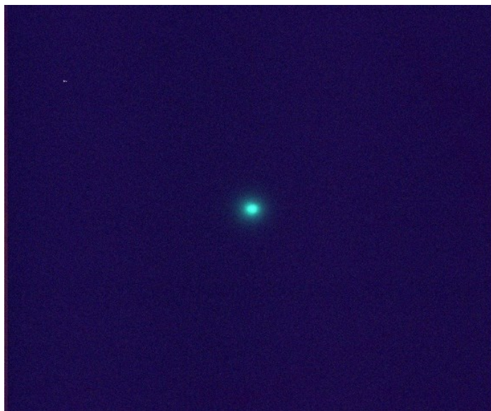
Figure 34: microscope image of the beam spot transmitted by a polycapillary lens at the focus distance.
