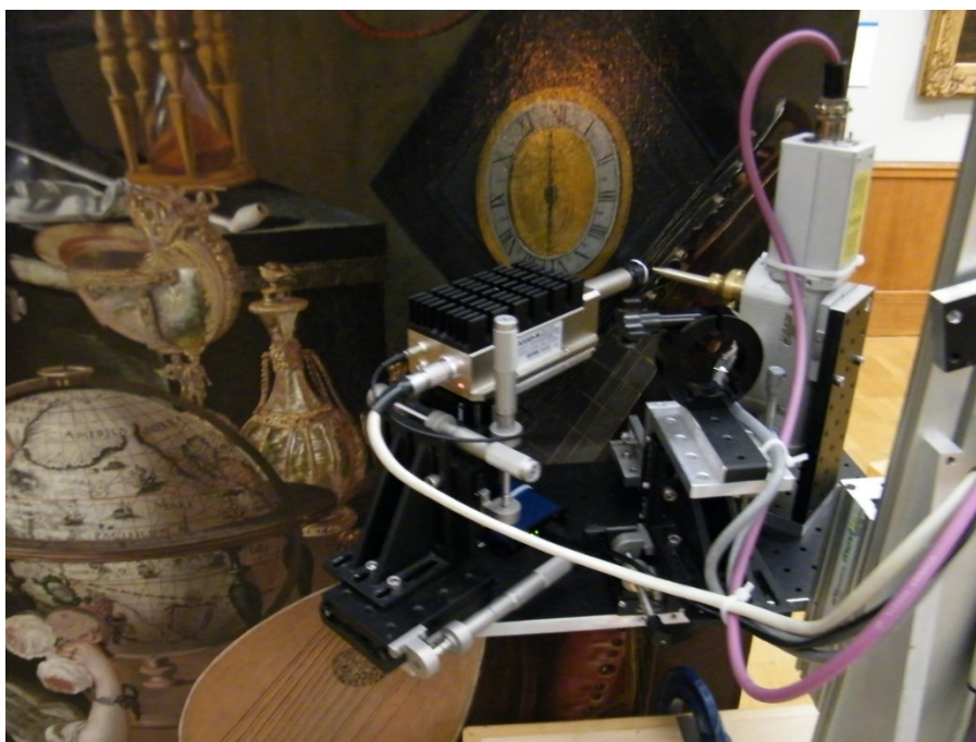
Figure 59: MA-XRF measurement on the Paston Treasure.
