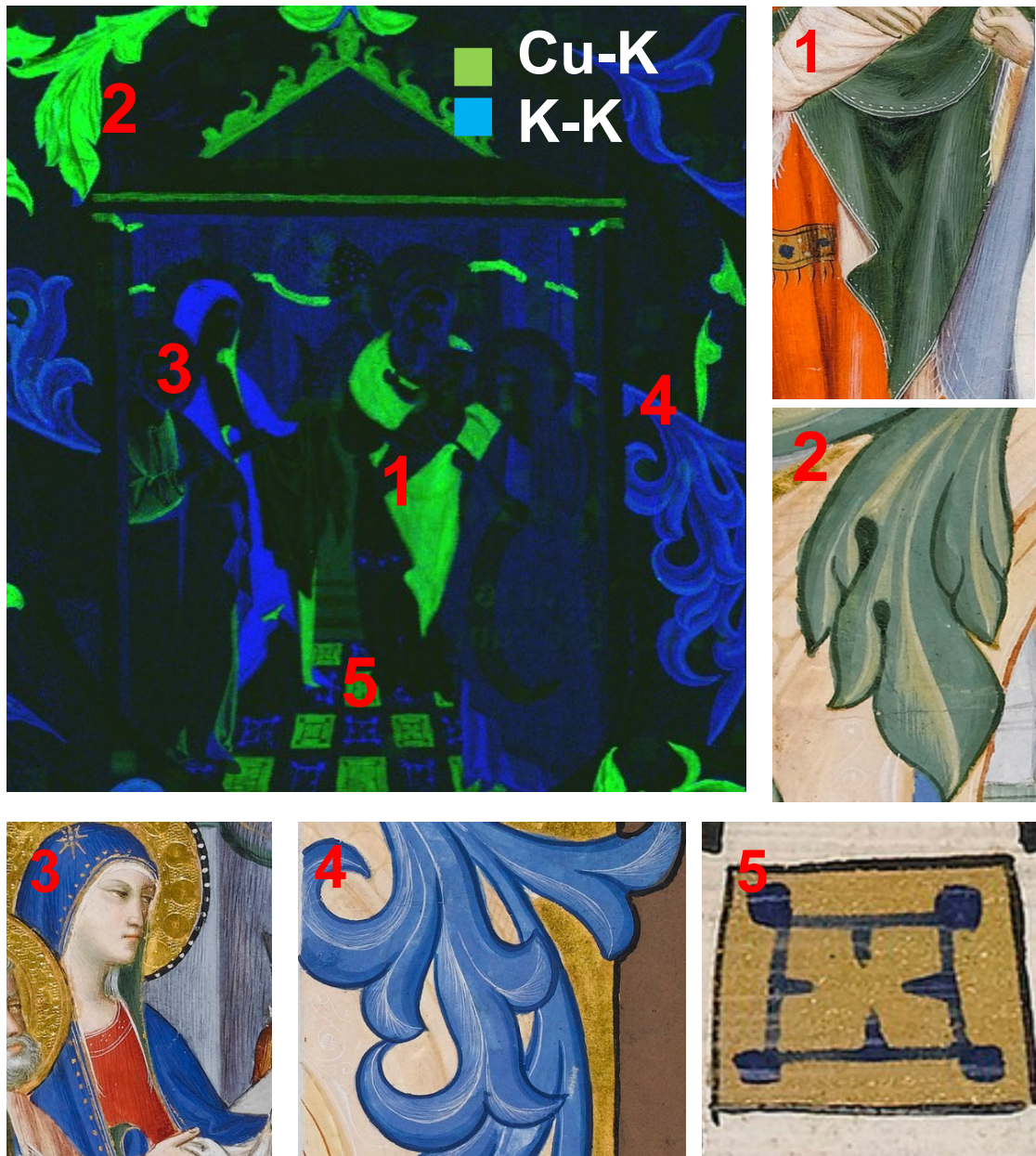
Figure 105: composite image Green: Cu-K – Blue: K-K and pictorial details characterized by copper (1-2) and potassium presence (3-5).
