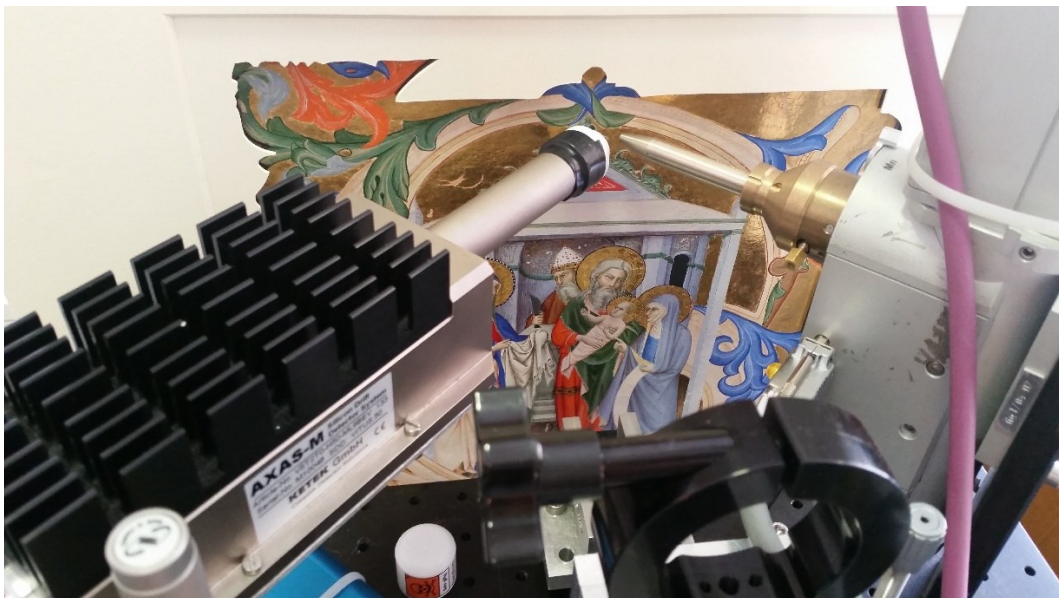
Figure 94: MA-XRF scanner installed at the Fitzwilliam museum
