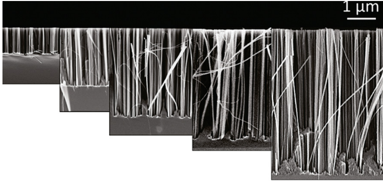
Figure 2.6: Cross section SEM images of Si NWs prepared by etching a (100)-oriented Si substrate covered by 2 nm of gold at different etching times. The length of the NWs are 1, 2, 3, 4, 5 \mu\text{m} respectively from left to right.
