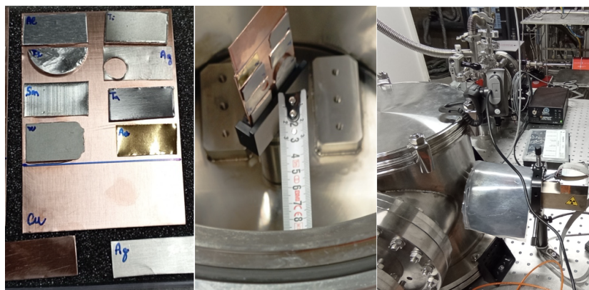
Figure 3.7: Multi-elemental target, consisting of a Cu plate with Al, Ti, Fe, Ag, Sn, Ta, W, Au smaller targets (left) - detail of the target mounted inside the vacuum irradiation chamber (middle) - external view of the irradiation chamber with the X-ray source on the right and the CCD camera at the back (right).
