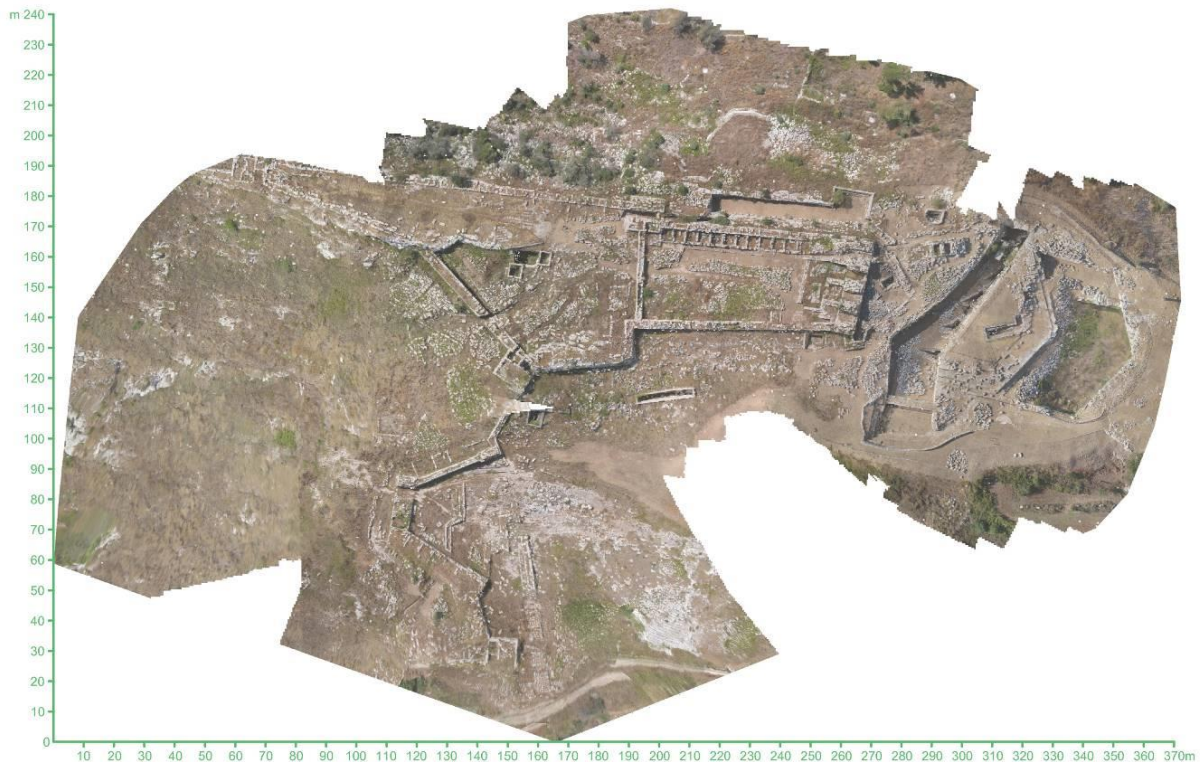
Figure 10. Orthophoto from TLS and UAS technology.
