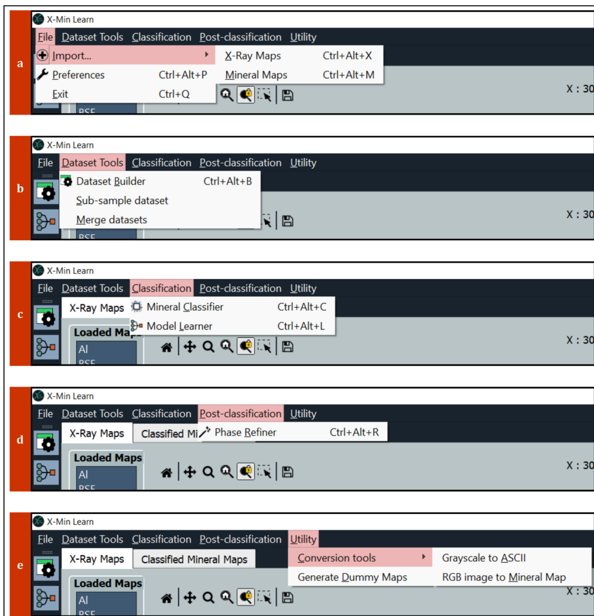
Figure S3.10 – Menu bar. (a) File menu, including import data options and preferences window (see Figure S3.11 ); (b) Dataset Tools menu, including the following tools: Dataset Builder ( Figure S3.14 ), Sub-sample dataset ( Figure S3.15 ) and Merge datasets ( Figure S3.16 ); (c) Classification menu, including the Mineral Classifier ( Figure S3.23 ) and the Model Learner ( Figure S3.17 , Figure S3.18 , Figure S3.19 , Figure S3.20 and Figure S3.21 ) tools; (d) Post-classification menu, including only the Phase Refiner tool ( Figure S3.29 and Figure S3.30 ); (e) Utility menu, including the Conversion Tools ( Figure S3.40 and Figure S3.41 ) and the Generate Dummy Maps tool ( Figure S3.42 ).
