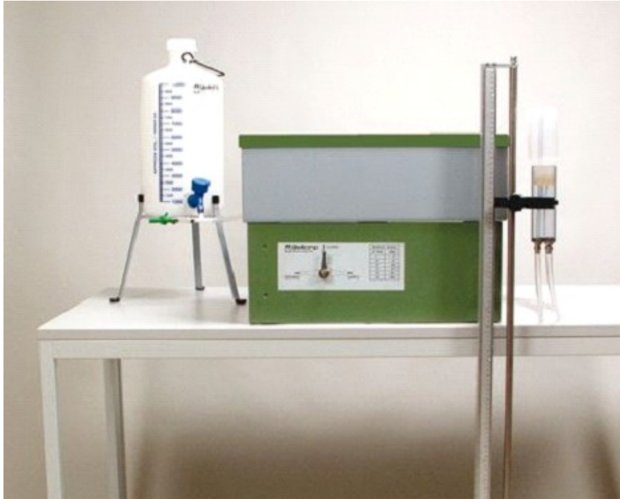
Fig. 4.24 Sanbdox for pF determination (Eijkelkamp).
