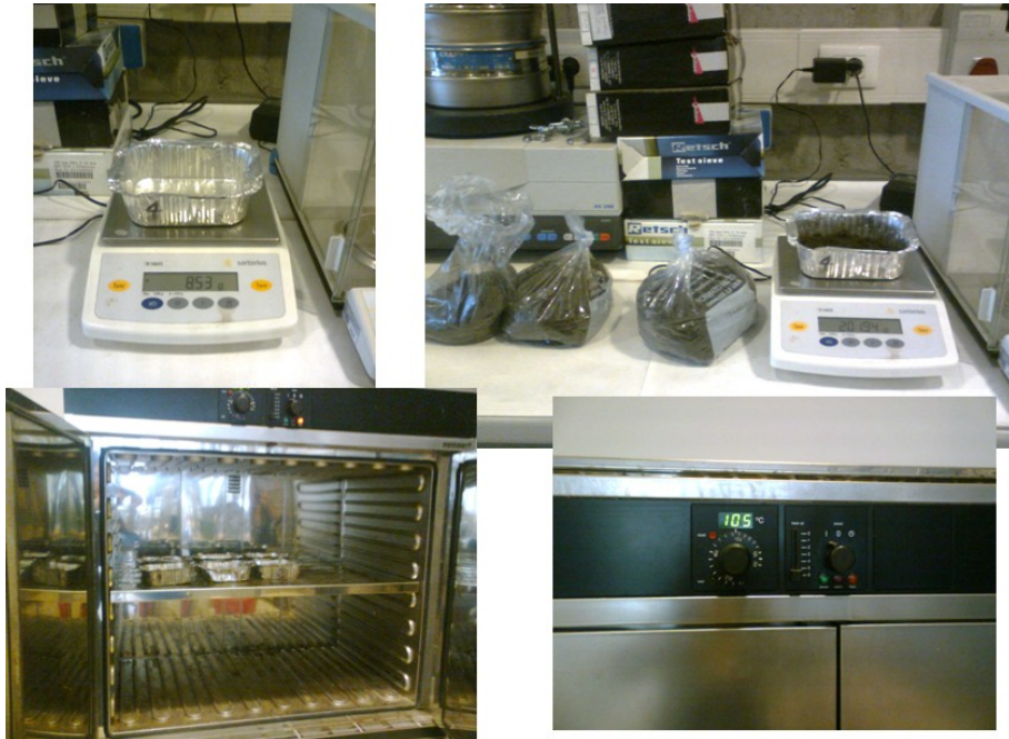
Fig. 4.28 Soil samples weighing and placement in a stove at 105 °C.
