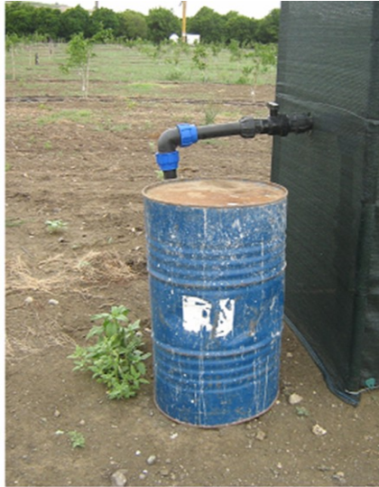
Fig. 4.17 Counters calibration in order to calculate the percentage error of the volumetric meters.
