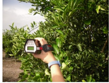
Fig. 4.35 Leaves temperature measurements (Everest 100szL).
