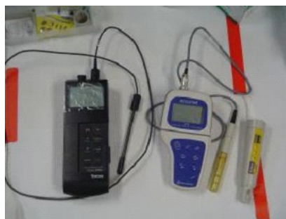
Fig. 4.19 Meters and probes to measure pH and electrical conductivity.
