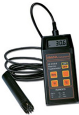
Fig. 4.36 Thermo hygrometer (HI 8564 – Hanna instruments), air temperature (°C) and humidity (%) measurements.
