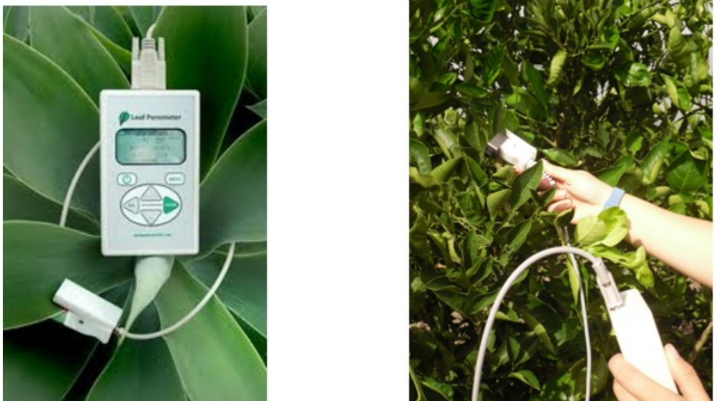
Fig. 4.34 Stomatal conductance (LP 80 – Decagon) measurements.
