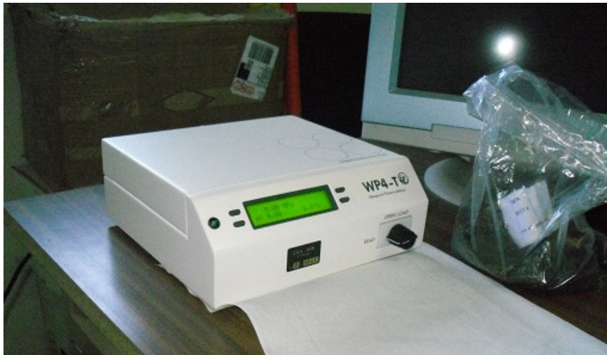
Fig. 4.27 Water potential measurement using psychrometer, WP4 (Decagon Devices)
