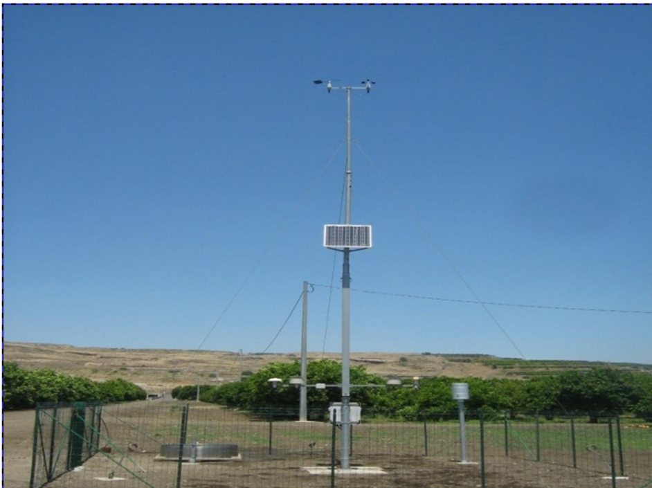
Fig. 4.4. Climate station and pan evaporimeter
