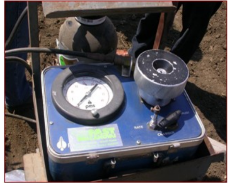
Fig. 4.30 Stem water potential (Scholander pressure chamber) measurement.
