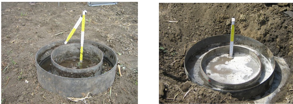
Fig. 4.22 Double ring infiltrometer.
