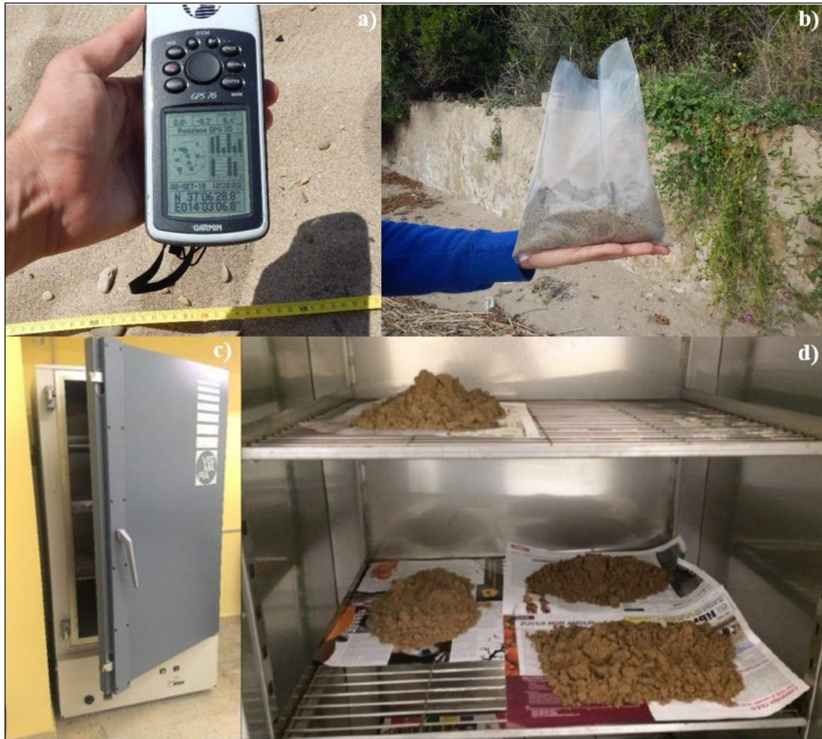
Fig. 51 – a) Garmin GPS 76S used to trace the position where the sediment samples have been collected; b) samples preserved in polythene bags; c) VISMARA Thermotop drying oven; d) dried sediment samples.
