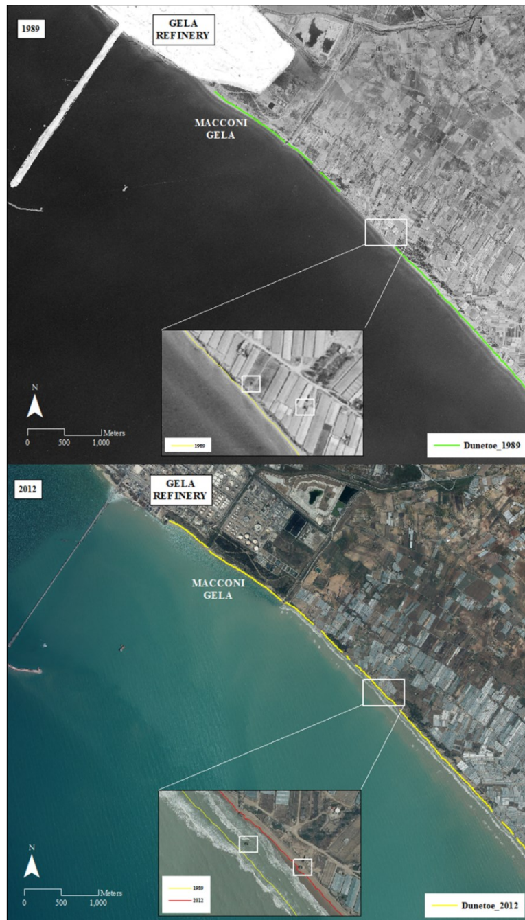
Fig. 68 – Significant shoreline and seafront dune ridge retreating between 1989 and 2012 are shown; within the two white squares manmade structures are framed, in 1989 they were on land, in 2012 they have been progressively swallowed up by the sea. Moreover, greenhouses and crop cultivations damage or destroyed the dune system whose fragmentation constantly increased over time.
