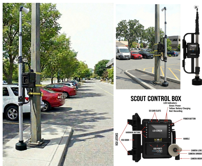
Figure 2. The MioVision Scout equipment and examples of deployment locations used for the field survey.
