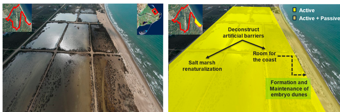
Figure 11. Illustrations from the plan to upscale coastal restoration in the northern part of the northern Ebro delta coast ( left , right inset), within the red line domain ( left inset). The picture also shows the proposed combination of active and passive restoration, combining enhanced coastal roughness (embryonic dunes) with the deconstruction of artificial barriers for coastal “room” ( right ).
