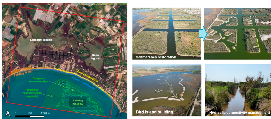
Figure 12. Some of the nature-based-solutions building blocks for the upscaled restoration plans in a set of lagoons in the Sicily pilot case ( left ), combining seagrass reconstruction ( left ), marsh restoration ( top right ), bird island building ( bottom left ) and hydraulic connectivity management ( bottom right ). Such systems, restored with the proposed upscaling (red line domain) for adaptation-through-restoration plans, provide gains in biodiversity and systemic risk reduction, enhancing natural and socioeconomic resilience under climate change.
