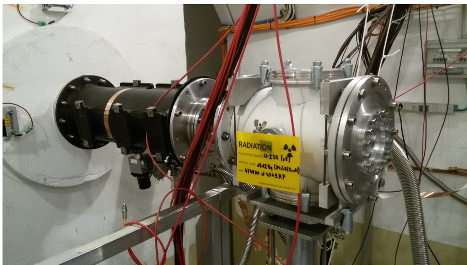
Figure 2.16: The experimental setup installed in the first n_TOF experimental area. The setup was contained in the aluminum reaction chamber, the neutron beam came from the wall on the left and reached the chamber traveling through the shown carbon fiber vacuum pipe.
