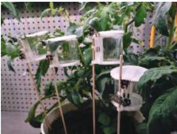
Fig. 2. Tomato plant with four clip cages demonstrating the clip cage design and experimental setup. Cage glass cylinder diameter and length are 46 mm and 40 mm, respectively.
