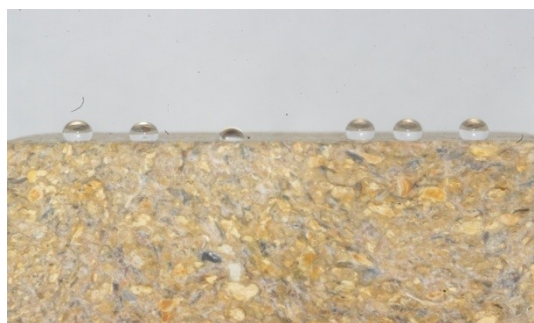
Figure 5.6 - Picture of water drops on WS3 coated Sabucina stone sample
