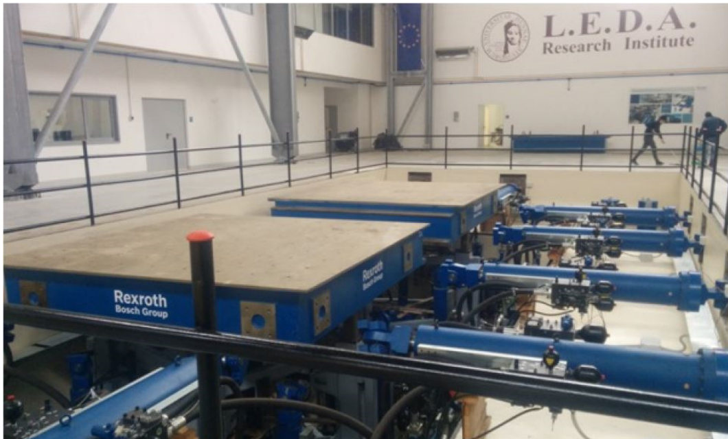
Figure 6.3 Photographic view of the shaking tables system (Navarra et al., 2015).
