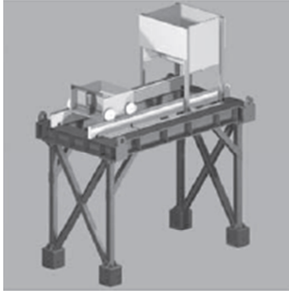
Figure 6.12 Schematic view of the pluviation equipment setup (Carvalho et al., 2010).
