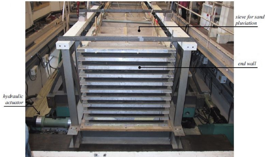
Figure 3.5 General view of the shear stack (From Biondi et al. 2015).
